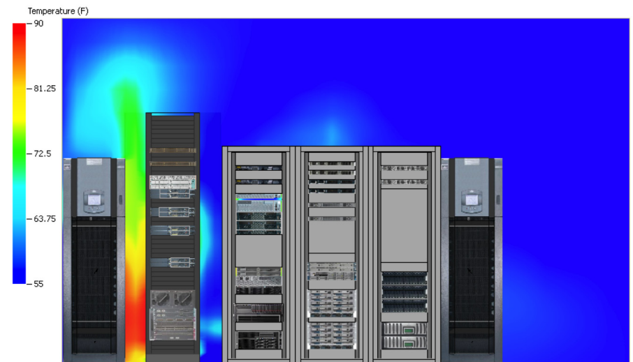
Figure 23 - Cross-sectional view of R1 temperature distribution through center line of rack
