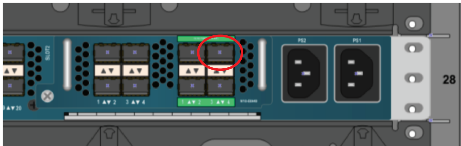
Figure 27 - Uplink a port on a UCS Fabric Interconnect
